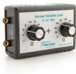
Figure 1. The Vernier Variable Load (VES-VL); the final series resistance is the sum of the two knob values (2–200 \Omega , max 0.3 A).
