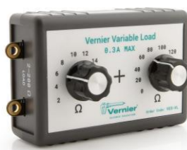
Figure 1. The Vernier Variable Load (VES-VL); the final series resistance is the sum of the two knob values (2–200 \Omega , max 0.3 A).
