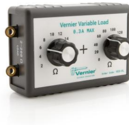
Figure 2. The Vernier Variable Load (VES-VL); the final series resistance is the sum of the two knob values (2–200 Ω, max 0.3 A).
