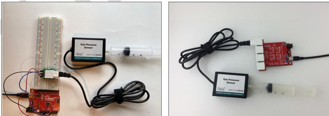
*Figure 1 Vernier Protoboard Adapter on a protoboard (l) and the Vernier Interface Shield (r)*
