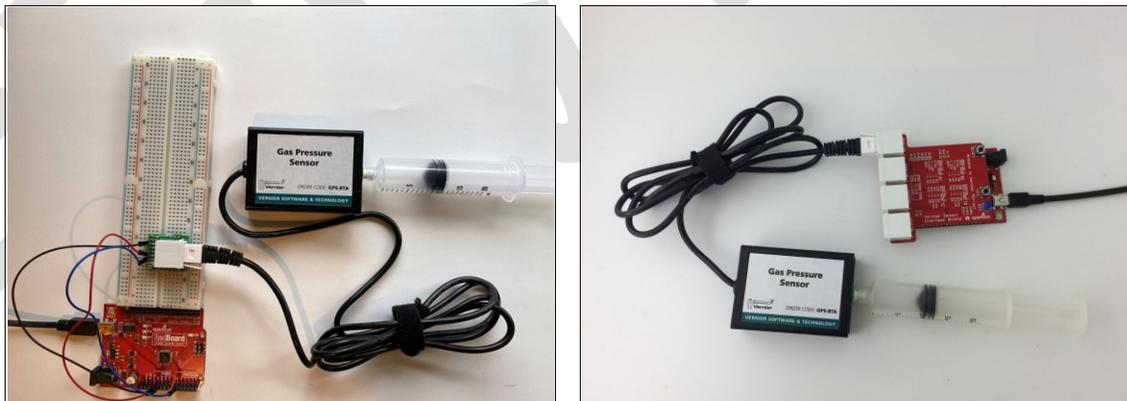
*Figure 1 Connecting a Vernier Gas Pressure Sensor to a Protoboard Adapter (left) and Interface Shield (right)*
